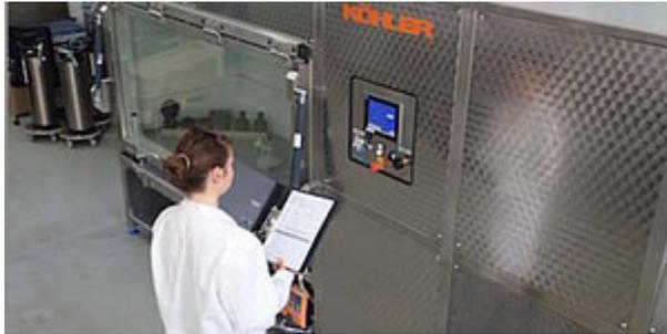
IGOS has expanded its testing equipment to include a universal testing chamber, which enables complete, uninterrupted corrosion testing in a single installation.
